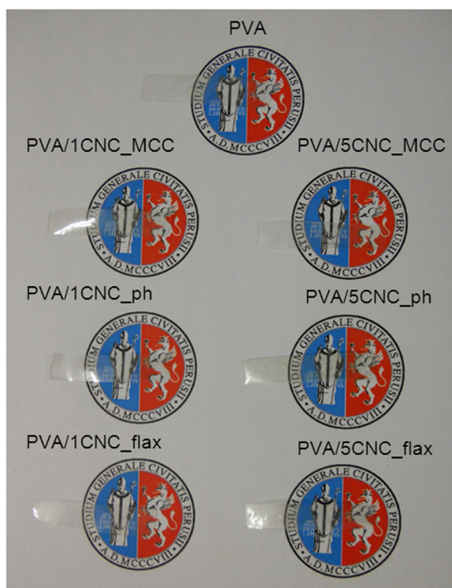
Fig. 4. Transmittance behaviour (Panel A), transmittance values at 700 nm (panel B) and visual observation (Panel C) of PVA and PVA bio-nanocomposites.
